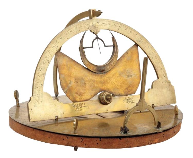
Facing page: Combined qiblah-compass and sundial, or 'equatorial circle' (*Da'irat Al-Mu*, addi), signed by its maker, 'Ali. Istanbul. Dated 1161 AH (1748-49). Beaten, cast and engraved brass attached to a wooden base. 17.3 x 24.2 cm (diameter). © Nour Foundation.
